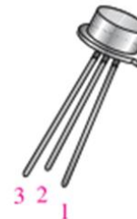
(c) TO-18. Emitter is closest to tab.
